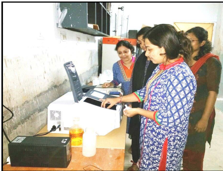
Fig 4.7: UV-Visible Spectrophotometer being used by students in the Central Instrumentation Facility Lab
